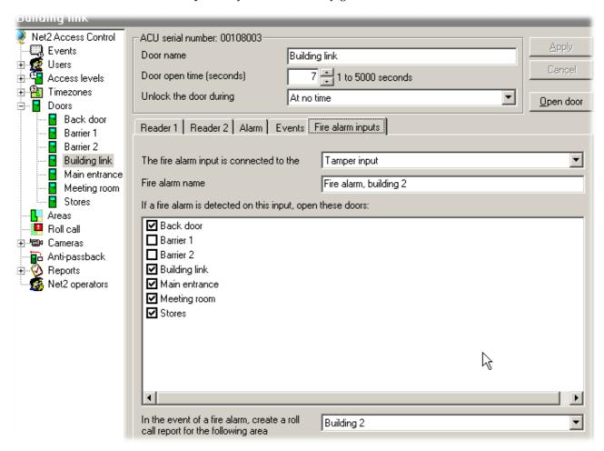
In this example, we have said that a normally closed output from the fire alarm system has been wired into the Tamper input (Between Tamper and 0V). If the fire alarm should go off, the Back door, Building link, Main entrance, Meeting room and Stores doors will open. In addition, a roll call report for Building 2 will be generated.
