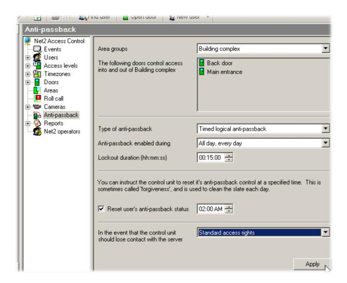
A door may not be on more than one anti-passback boundary. For instance, if you set up anti-passback for the **Building complex**, you would not be able to also have anti-passback on **Building 1**, because the Main entrance would then be used twice. You could, of course, have anti-passback control on the car park as well as on the Building complex, as there are no conflicts of reader.
