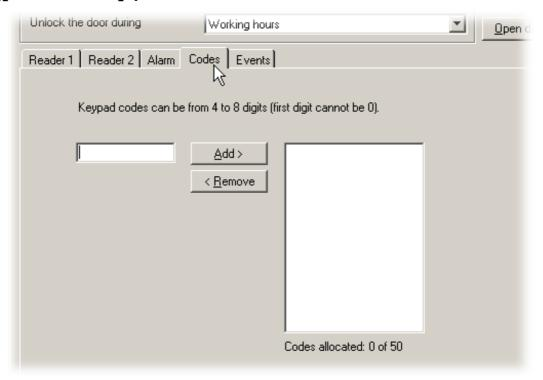
Note: The Codes tab only appears if a keypad is configured on the control unit.
