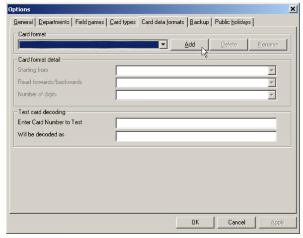
The Net2 system identifies users by reading an 8 digit number from their user card/token. Each user has to have a unique number for the system to recognise them. If cards other than the Net2 cards are used, only a portion of the data on the card may be unique. It is possible to configure the Net2 system to look at the unique part of the card information.
