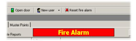
You can either click on the 'Reset fire alarm' button on the toolbar, or alternatively, double click the alarm event from the event view. Either of these acknowledges the fire alarm, and closes any fire doors that may have opened.
