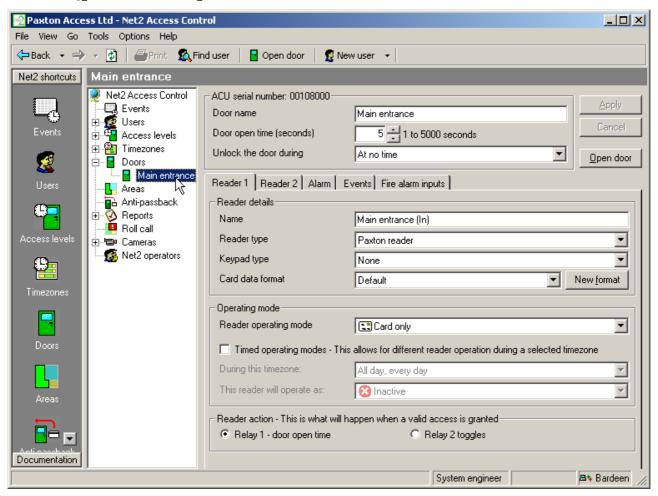
The settings for each control unit are configured in this screen. The ACU serial number is shown in the top left corner of the main display. The lower section of the main display has tabs that allow access to the different settings (Reader1, Reader2, Alarm, Codes and Events). Sections are accessed by clicking on the relevant tab.
