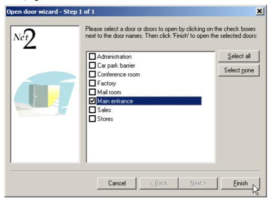
The open door wizard can be accessed from the toolbar at the top of the screen. Any doors on the system can be made to open for door open time from the software.
