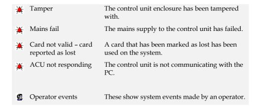
If the PC is switched on, events will be reported almost immediately. If the PC is switched off the event will be held at the control unit (2,300 event buffer) until the PC is next switched on.
