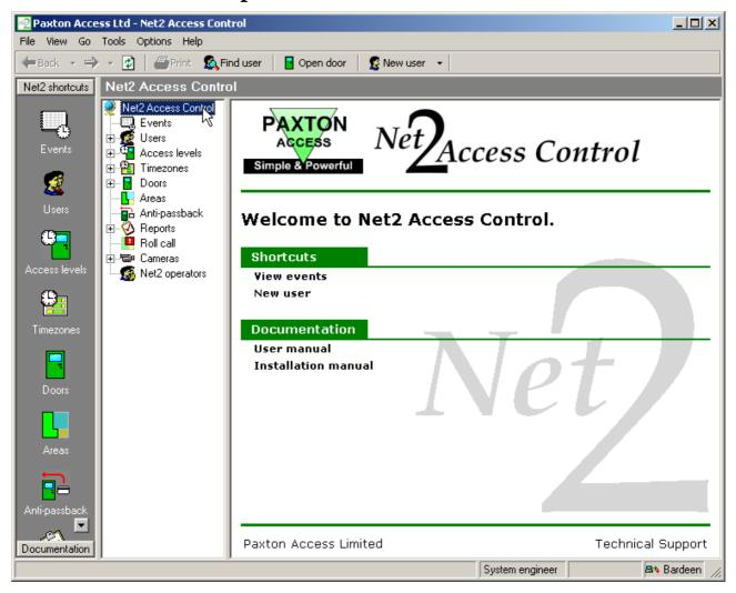
The screen shot shows the three windows of the Net2 software. In addition to these windows there are drop down menus and a task bar.
