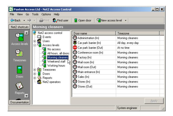
Every reader on the system is displayed. Next to the reader name, a timezone can be selected from the drop down menu. When a user is given an access level, they will be permitted through the readers shown, during the timezones shown.
