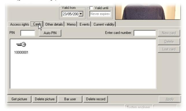
The main display shows the cards that are assigned to the user. As many cards as required can be assigned to a user (the overall system limit is 10,000 cards). Cards can be added by either entering the card number manually OR by presenting or swiping the card at the desktop reader. Cards can be deleted completely by pressing the **Delete card** button.
